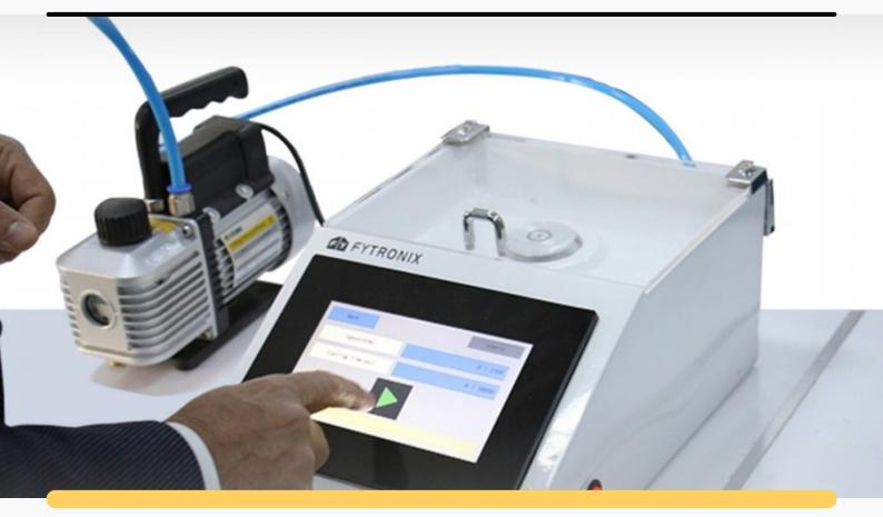
This spin coater coat the organic materials and metal oxides and all-in solutions. The spin coater is a complete solution coating system.
