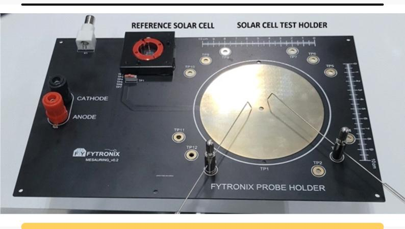
This holder can be used to measure current voltage characteristics of the solar cell
