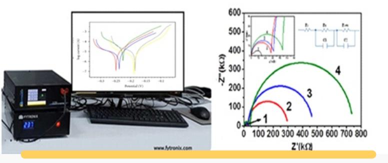
System includes Impedance ANALYZER Nyquist characteristics (real and d imaginary impedance) Frequency range: 1 mHz-10 MHz Sourcemeter Voltage range. -20 V to 20 V or more (negative and positive voltages) Current range: 1 nA-500 mA Current-voltage characteristicss
