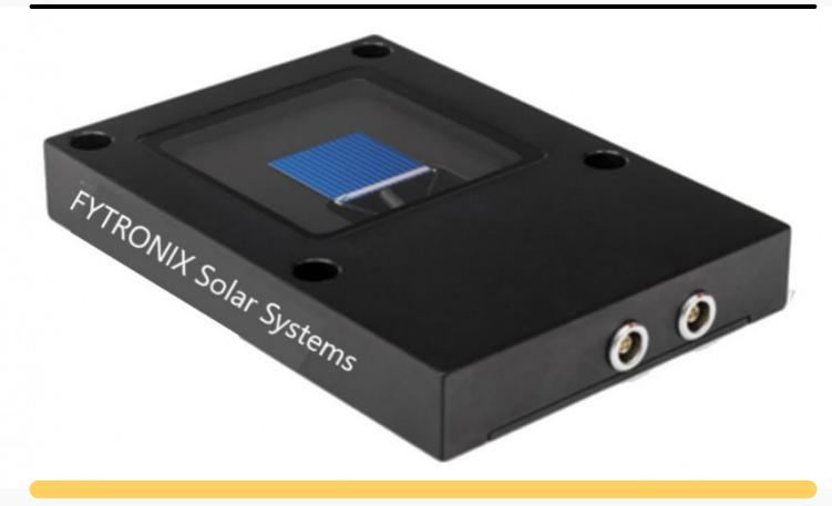
The reference cell is used for the determination of solar simulator irradiance levels. FYTRONIX uses it to calibrate the solar cells indoor. The calibration is done against an established set of reference cells calibrated at NREL These references are measured each year at the International Spectroradiometer Intercomparison (ISRC) to ensure trace-ability. This all results in a lower cost reference cell that is very well suited for indoor applications.
