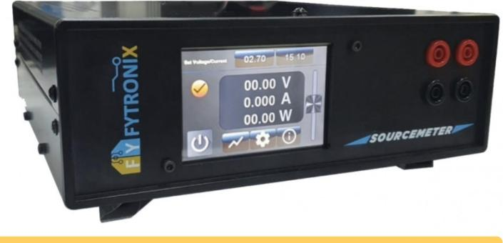
FY 8000 Sourcemter measures current-voltage (I-V) characteristics of solar cells, Schottky diode, p-n junction, photosensors, biosensor, gas sensors under various external effects.
