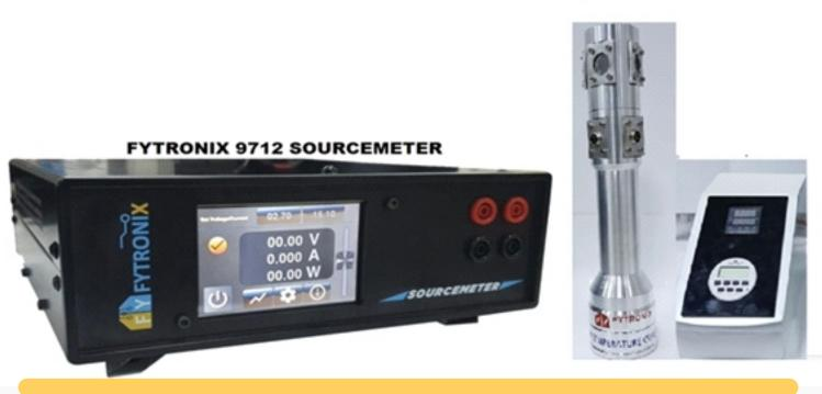
System measure electrical conductivity of semiconductor, organic semiconductor, superconductor and metals as a function temperature.
