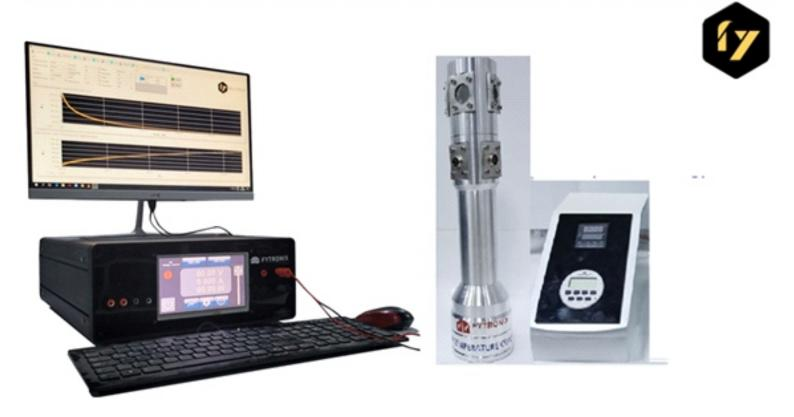
System measure AC conductivity and dielectric parameters of powder and thin film materials. System have software for measurements of all dielectric parameters and AC conductivity parameters of powder sample and thin film samples at variable frequencies as a function of temperature and a part of software for analysis of the results.
